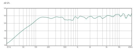
This graph shows the frequency response for a 1-watt swept sine signal in an anechoic environement (4pi), measured at 3 m and scaled down at 1 m
